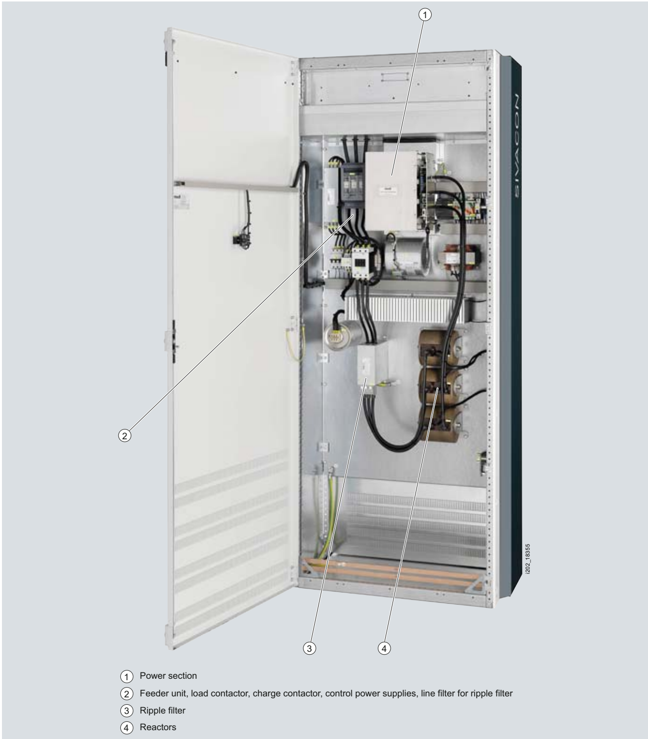
Filter module 4RF1010-3PB0
